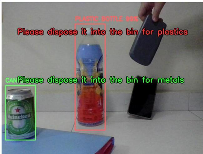
The image below shows all three recyclables detected at once. The rectangular boxes and text are colour-coded to not confuse users when there are too many recyclables on screen at once.
