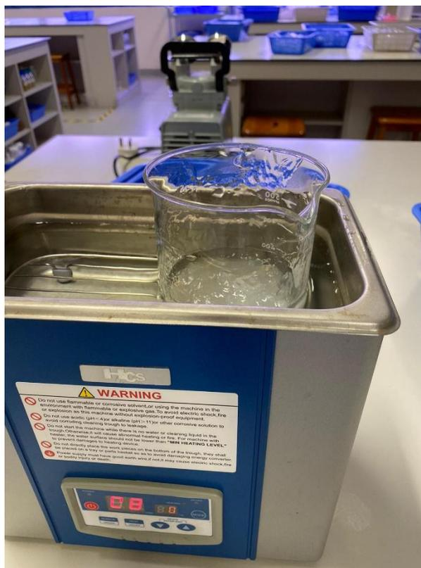
**Fig. 4 Ultrasonic bath sonicator**
