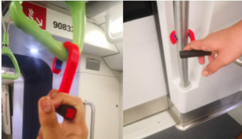
Fig. 6 showing our device used for latching onto hand straps in MRT trains
