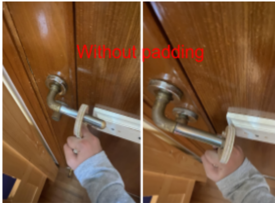
Fig. 4a showing the position of hook before pulling it down
