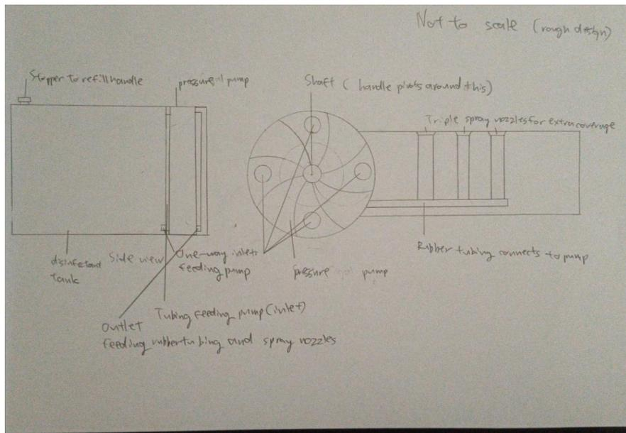
This is one of our drawings. The left-hand side drawing is the side of the door handle which will be hollow to contain the disinfectant and also will have a stopper to refill. There is a one-way inlet to take in the disinfectant from the storage area when the door handle is pushed back. The inlet is then linked to the four tubings.
