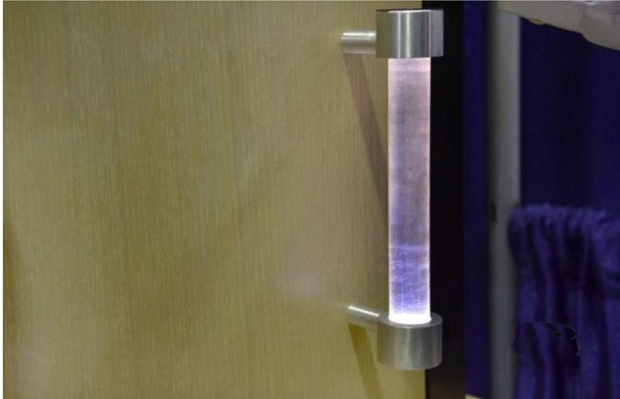
This is a self-sanitizing door handle made by two university students. There is a power generator inside the door handle which converts the kinetic energy produced when the door is being opened into electrical energy. Then, UV light is activated, causing a chemical reaction in the chemicals on the glass tube to kill all bacteria and viruses living on the door handle.
