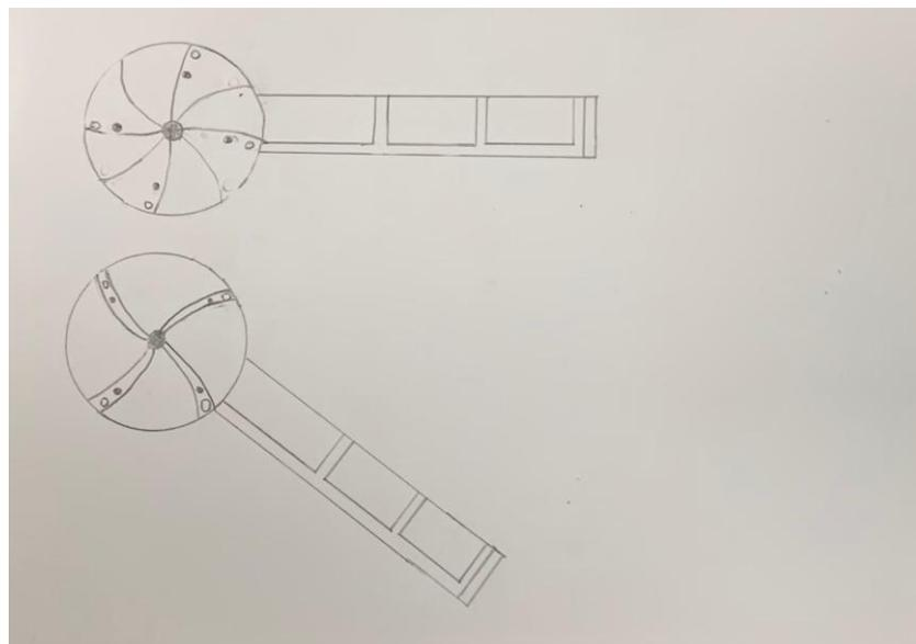
The tubings will then be connected to the pump as represented by the shaded circles at the back of the pump, which the blades are made up of metal with rubber coating and the case itself is made up of stainless steel. The one-way outlets, at which are represented by unshaded circles on the top of the casing will be connected to four pipes that later joins together and connects to the three spray nozzles that will squirt out the disinfectant.
