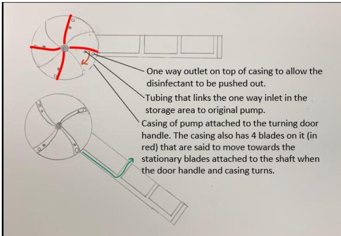
When the handle is pushed downwards, the casing attached to the handle will also turn, bringing the four blades towards the other four stationary blades. This increases the pressure in between the blades, pushing the disinfectant out from four one-way outlets on the top of the casing. Then the disinfectant will flow into the rubber tubing system connected to the outlets (not drawn) and out of the three spray nozzles to sanitize the user's hand and at the same time disinfect the door handle.
