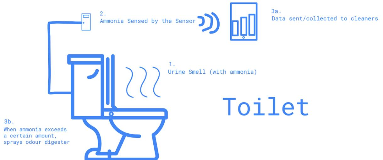
The illustration of our product shows how the product is placed in the toilet and how it will be able to detect the ammonia levels in the toilet and how the odour digester will be deployed when ammonia levels exceed a certain amount. The illustration shows how the system is connected and the possible issues such as dirt and inaccessibility where the sensor is placed.
