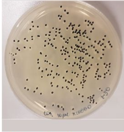
Figure 2: Soaking test result for conventionally-synthesised silver nanoparticle solution setup, visible colonies labelled with marker
