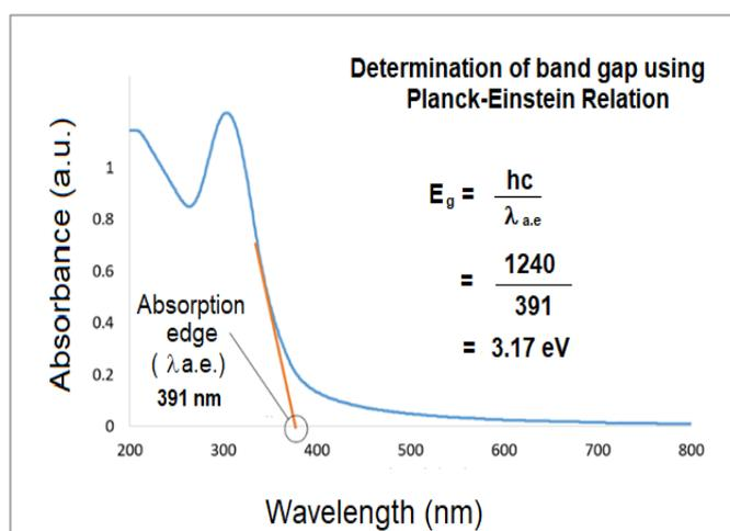
Figure 6: UV-Vis spectrum of  $K_2W_4O_{13}$  nanowires for use in calculation of band gap
