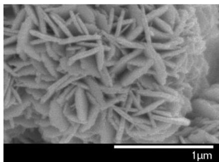
Figure 1: SEM image of K<sub>2</sub>W<sub>4</sub>O<sub>13</sub> nanowires
