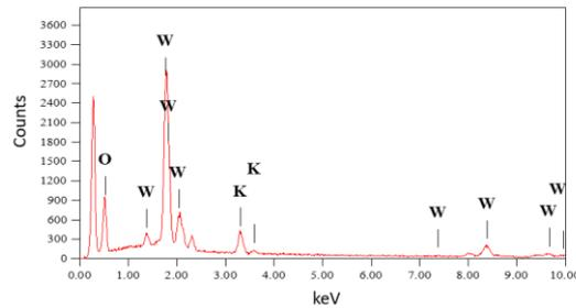
Figure 2: EDS of  $K_2W_4O_{13}$  nanowires synthesized
