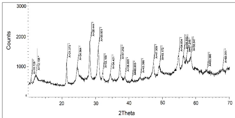
Figure 3: XRD pattern of  $K_2W_4O_{13}$  nanowires synthesized
