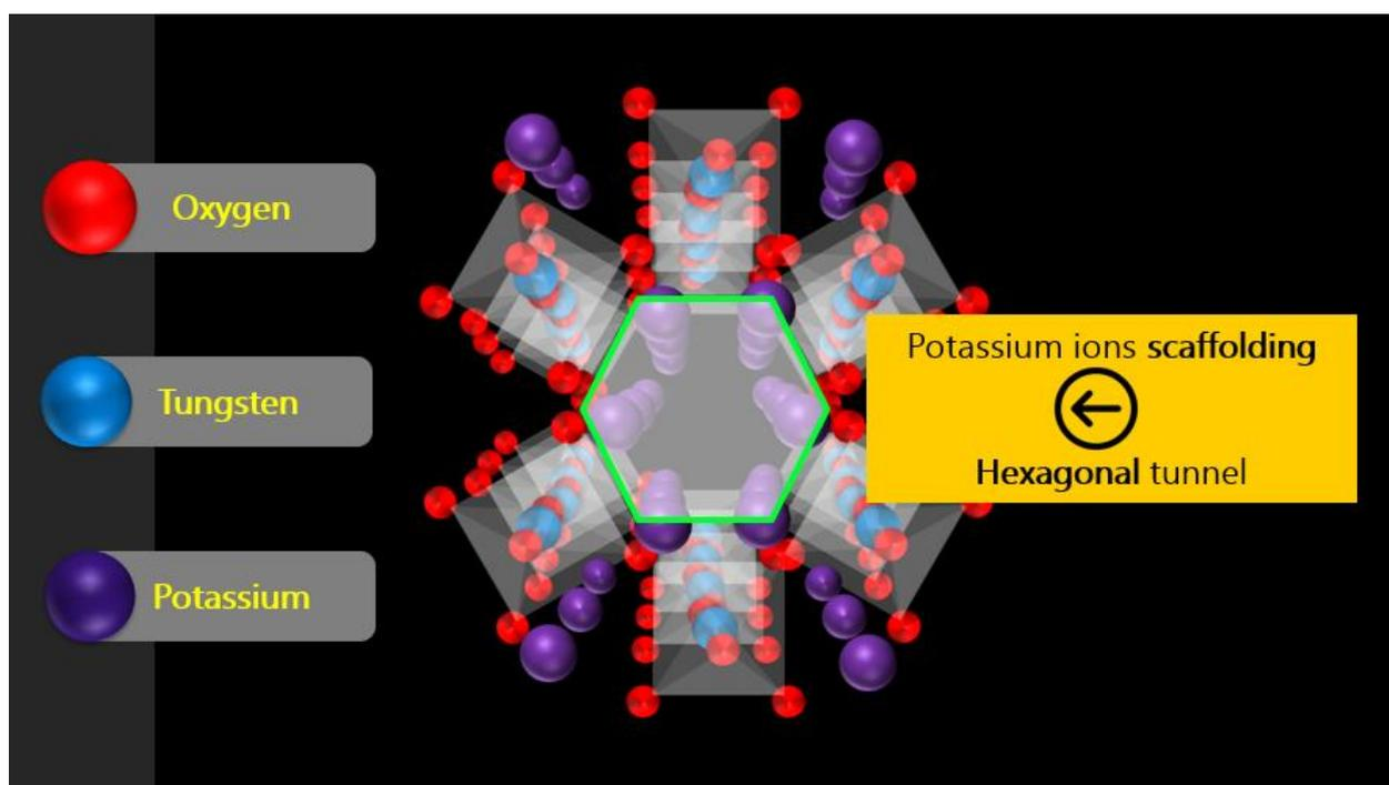
Figure 14: Structure of  $K_2W_4O_{13}$  nanowires
