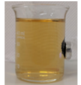
Figure 6: Magnetic attraction of adsorbent for separation
