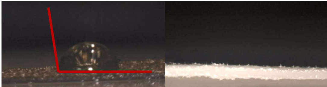
Figure 2: Underoil contact angle measurement of water on PDA-coated filter paper (left) and unmodified filter paper (right)
