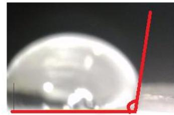
Figure 4. How water contact angle is measured
