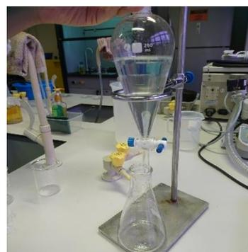
Figure 6. Extraction of remaining diesel using hexane and a separating funnel
