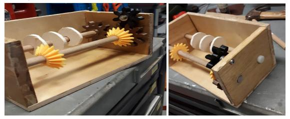
When the crank is turned, the two brown gears at the back will turn, therefore spinning both shafts. The cams on the second layer power the skyscrapers rising and falling; the two gears in the first layer allow the ferris wheel to be set up and spin; the two bevel gears will power the boat using another mechanism.
