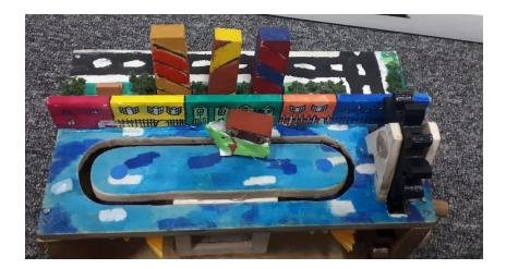
We had to cut the wood in openings where the skyscrapers rise and fall, the path of the boat, and below the ferris wheel. By working closely with the SRC laboratory assistants, Mdm Chua and Mdm Foo, we were able to cut it open at the desired locations. After doing that, we painted the cover and added artificial grass along the roads, before nailing it on top of the automaton.
