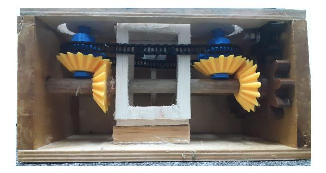
4 bevel gears interlock with each other to transmit rotary motion from the horizontal crankshaft to the blue vertical shafts. The vertical shafts have a stopper on them to prevent the bevel gears from slipping down and away from their positions. This
