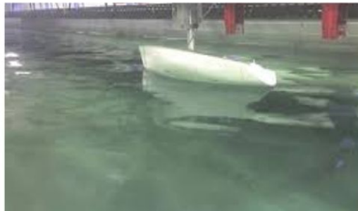
Figure A.1 Model ship resistance coefficient testing
