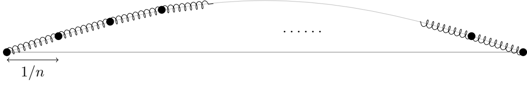
Figure 2: A finite difference approximation with (n + 1) point masses.
