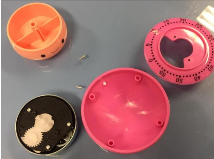
Initially, the invention was designed to not be battery operated. However, this proved impractical as the mechanical energy provided by the ending of the DAISO timer was insufficient to move the knob of the stove.
