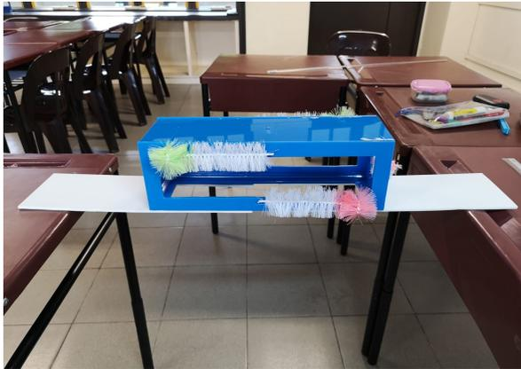
Therefore, we bought affordable brushes from a provision shop and found the other materials we needed from Makerspace, namely six 5mm cast acrylic sheets and one 3mm cast acrylic sheet. In order to build the prototype itself, we made our way to the Science Research Centre Physics Lab to use the scroll saws, hole drills, files and chloroform to cut out necessary pieces of the plastic and assemble our prototype with the supervision of the teachers there.
