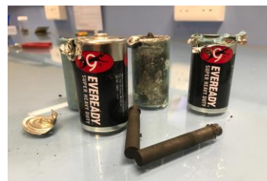
Figure 2: Graphite rods extracted from used zinc carbon batteries
