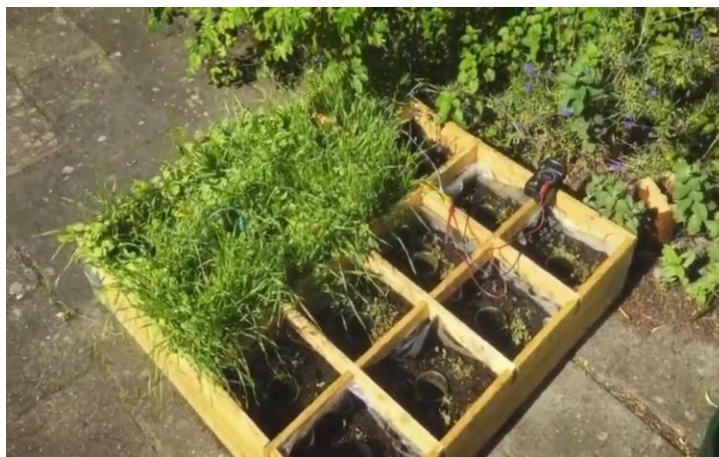
Figure 21: Application of MFC in garden to power LED lights and plant-watering sensors
