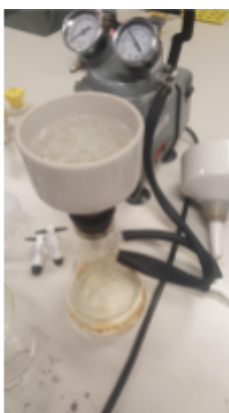
Figure 3 :Vacuum filtration to remove water
