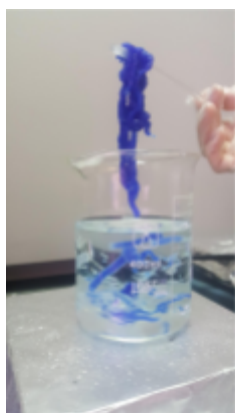
Figure 2 :Cellulose that precipitated
