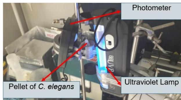
Figure 6: Light intensity measurement set-up
