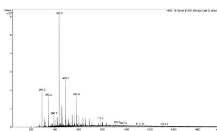
Figure 8: Mass spectrum of Sample B, right-most peak of 1319.2
