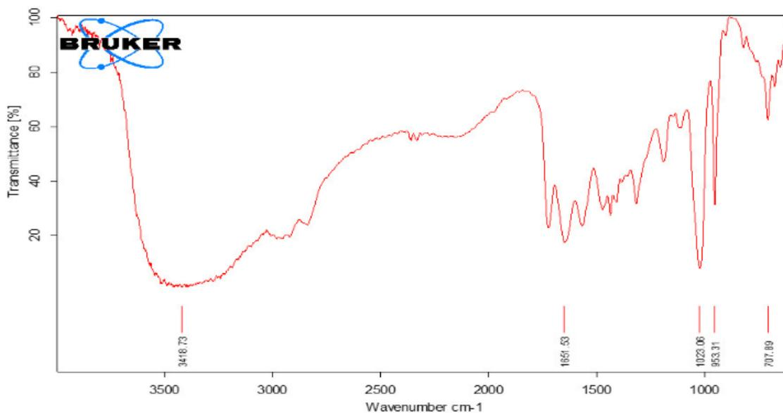
Figure 7: Fourier Transform Infra-red spectrum of HPBAE
