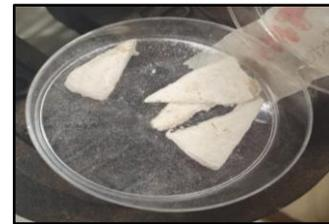
Figure 6. Titanium dioxide-coated cellulose aerogel.
