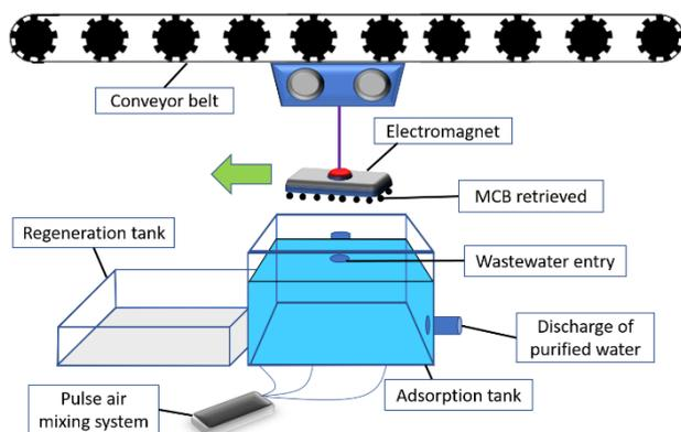
Figure 16: Proposed model for use of MCB in wastewater treatment plants
