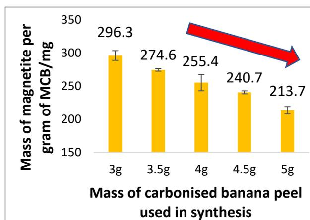
Figure 11: Mass of magnetite coating in MCB (3g) to MCB (5g). N=3
