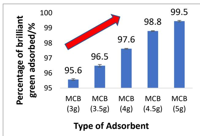
Figure 10: Adsorption of brilliant green by MCB (3g) to MCB (5g). N=5
