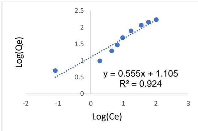
Figure 20: Freundlich isotherm for carbonised banana peel
