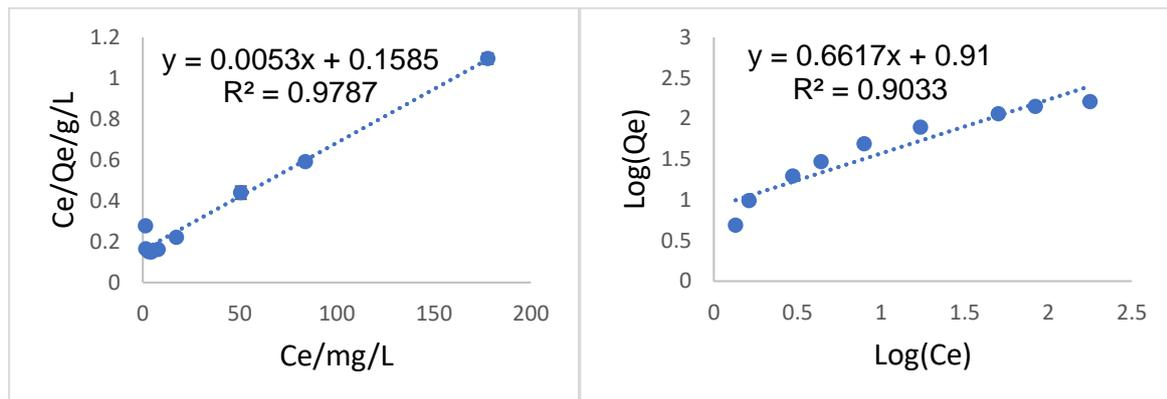
Figure 17: Langmuir isotherm for MCB
