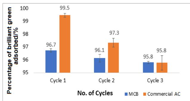
Figure 14: Regeneration of MCB and Commercial AC for re-adsorption of brilliant green. N=5
