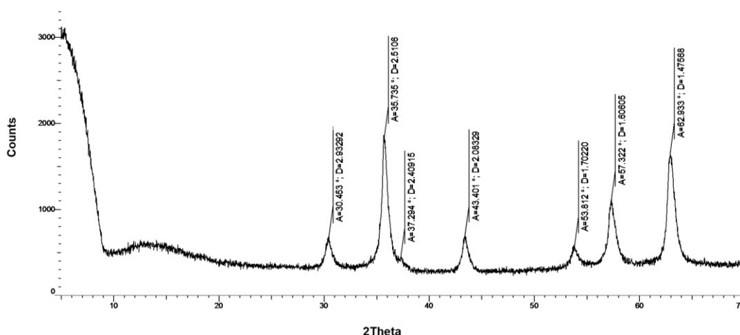
Figure 5: XRD spectrum of MCB (3g)
