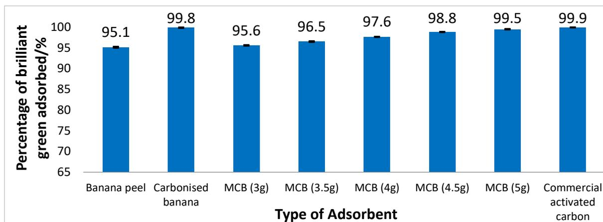
Figure 9: Adsorption of brilliant green by different adsorbents. N=5
