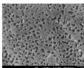
Figure 2: SEM image of carbonised banana peel
