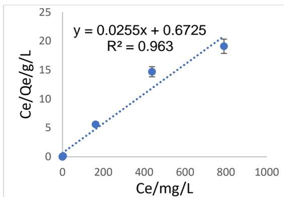
Figure 27: Langmuir isotherm for commercial AC
