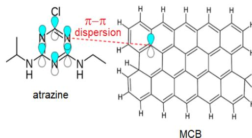
Figure 8: Proposed mechanism of how MCB adsorbs atrazine
