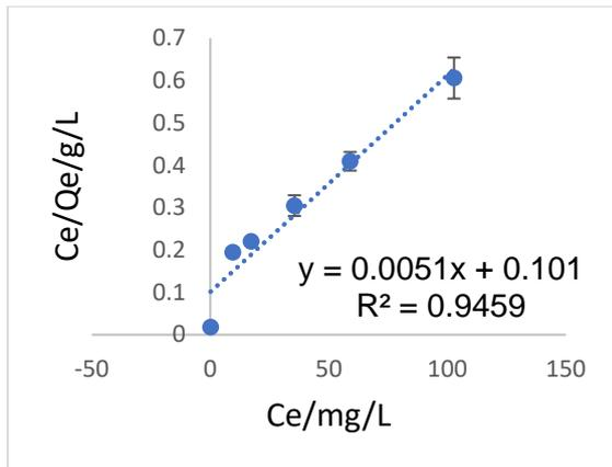
Figure 19: Langmuir isotherm for carbonised banana peel
