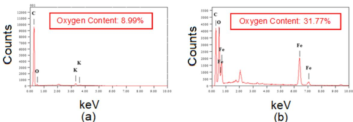
Figure 13: EDS of (a) Commercial AC and (b) MCB (3g)
