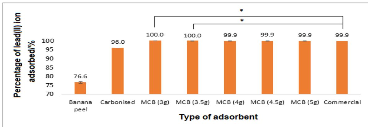
Figure 12: Adsorption of lead(II) ions by different adsorbents. \* denotes significant difference based on Mann-Whitney U test at significance level of 0.05. N=5
