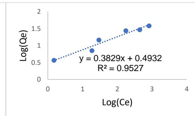
Figure 26: Freundlich isotherm for carbonised banana peel
