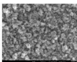
Figure 3: SEM of magnetite
