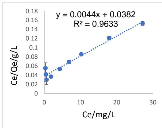
Figure 21: Langmuir isotherm for commercial AC
