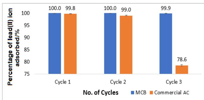
Figure 15: Regeneration of MCB and Commercial AC for re-adsorption of lead(II) ions. N=5
