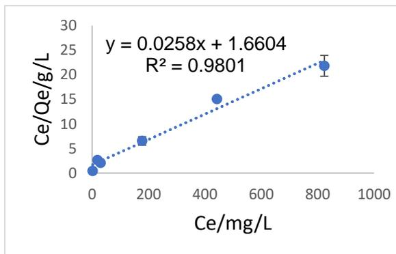
Figure 25: Langmuir isotherm for carbonised banana peel
