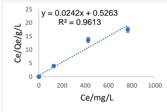
Figure 23: Langmuir isotherm for MCB
