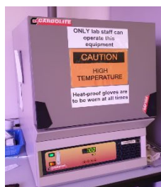
Figure 3. Calcining eggshell in a furnace
