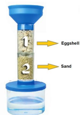
Figure 19. Filter containing eggshell for water purification
