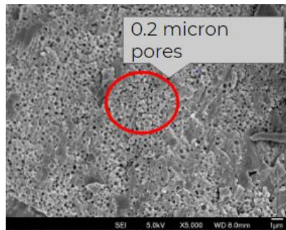
Figure 6. SEM image of eggshell powder
