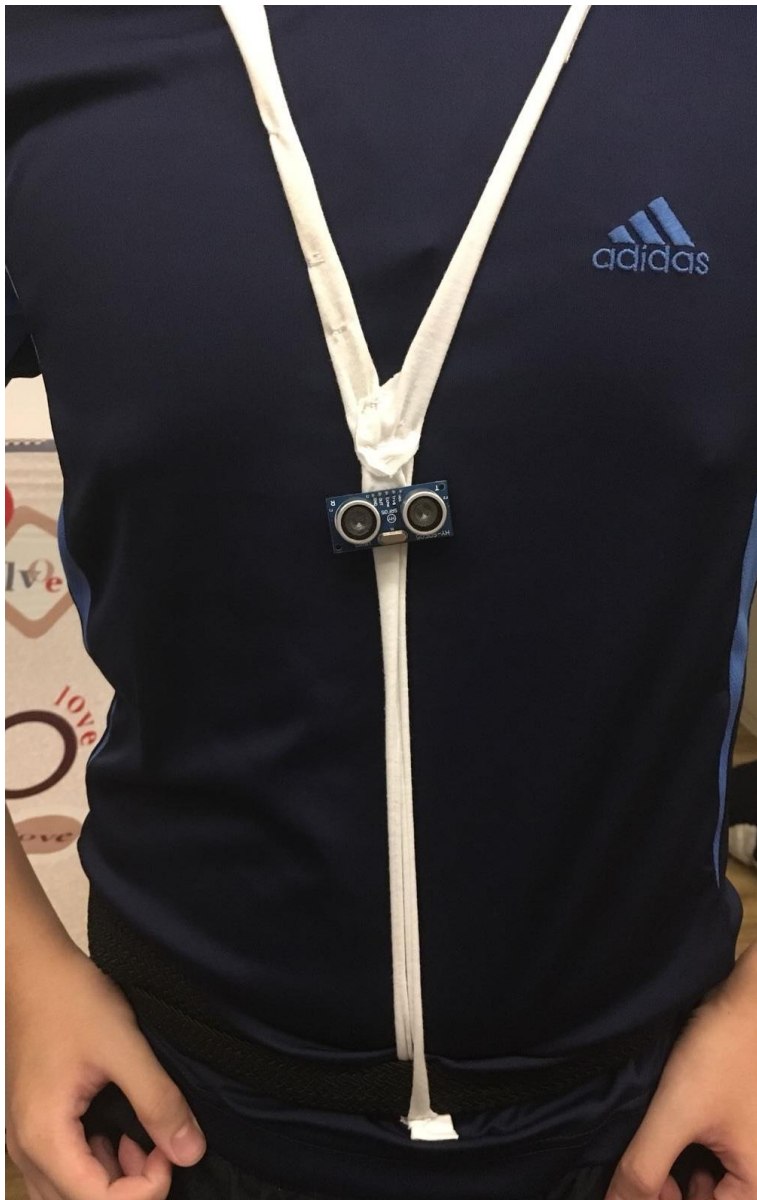
Figure VIII Front View (Worn), only the ultrasound is found on the front of the person's chest, this is to ensure that the ultrasound is as near to the chest as possible, increasing accuracy of ultrasonic sensor.
