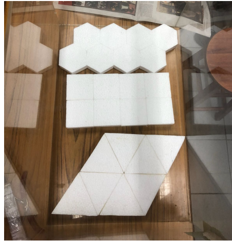
Fig 1. Foam floating structures made from 8 modules each, with different module shapes (from top: hexagonal, square, triangular)
